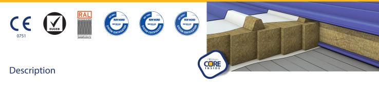
**FIBRAN***geo* **CORE BL-50** is produced from molten mineral rock, initially fused in an electric furnace at more than 1500°C and then spun into fibres. The loose stonewool fibres, with the addition of adhesive resin, oil and special compounds that provide water repellency, become cohesive, elastic, non-hygroscopic and water-repellent. Fibres are formed in boards and cut to size as required by application. Products are finally shrink-wrapped in PE film and packed on pallets.
