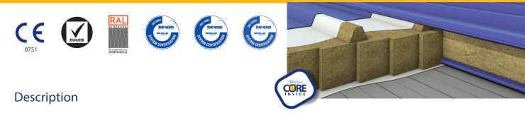
**FIBRAN***geo* **CORE BL-40c** is produced from molten mineral rock, initially fused in an electric furnace at more than 1500°C and then spun into fibres. The loose stonewool fibres, with the addition of adhesive resin, oil and special compounds that provide water repellency, become cohesive, elastic, non-hygroscopic and water-repellent. Fibres are formed in boards and cut to size as required by application. Products are finally shrink-wrapped in PE film and packed on pallets.
